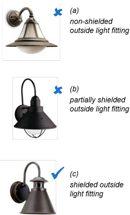
Figure 4 Shielding characteristics of light fittings
